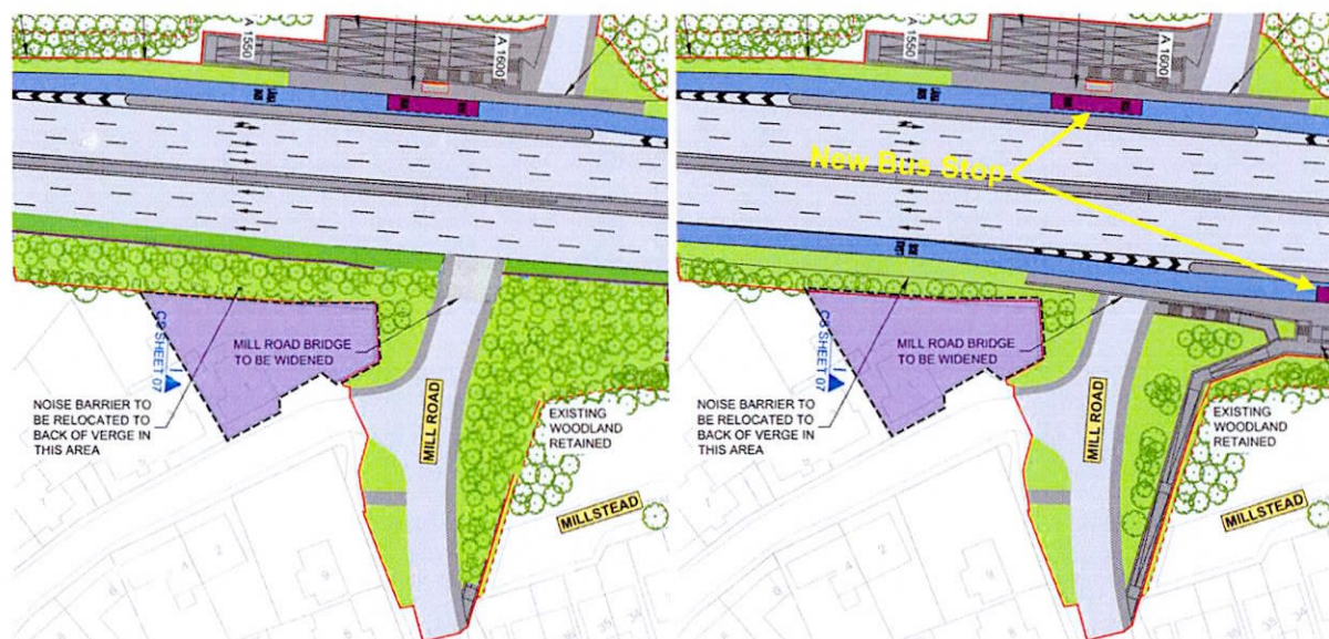
Figure 4.0 Extracts of Sheet 10 of the General Arrangement drawing illustrating the existing situation (l) and proposed works (r) relative to our client's site.
